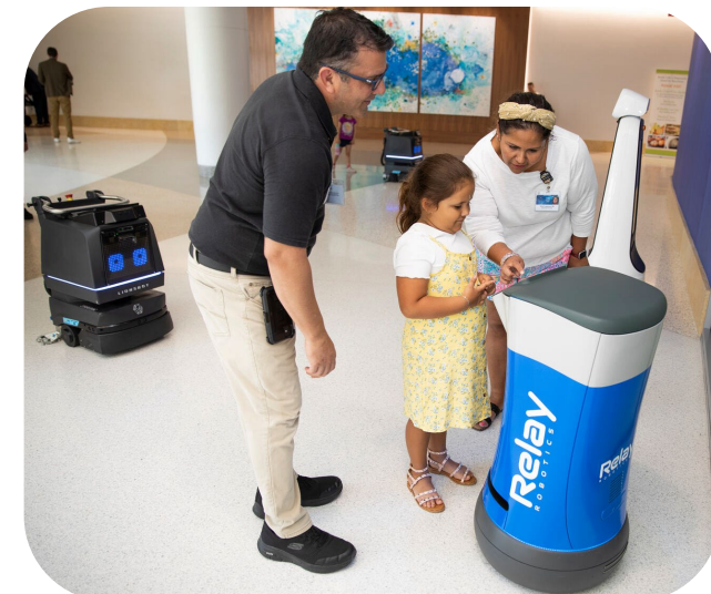
FIGURE 1: Floor cleaning robot (left) and supply delivery robot (right)
